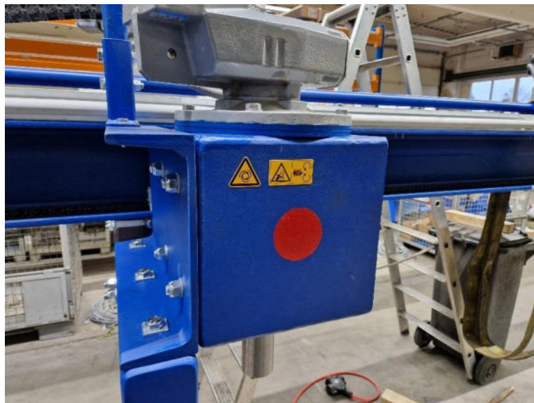
Figure 13: Put the red auger on the side with the red point
