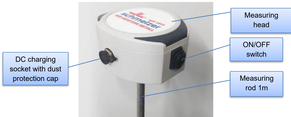
Figure 7: Measuring head overview
