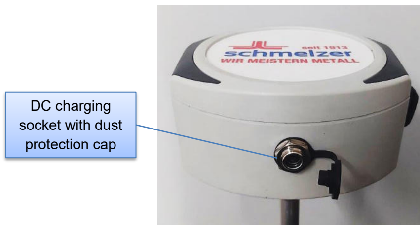
Figure 8: Open DC charging socket.
