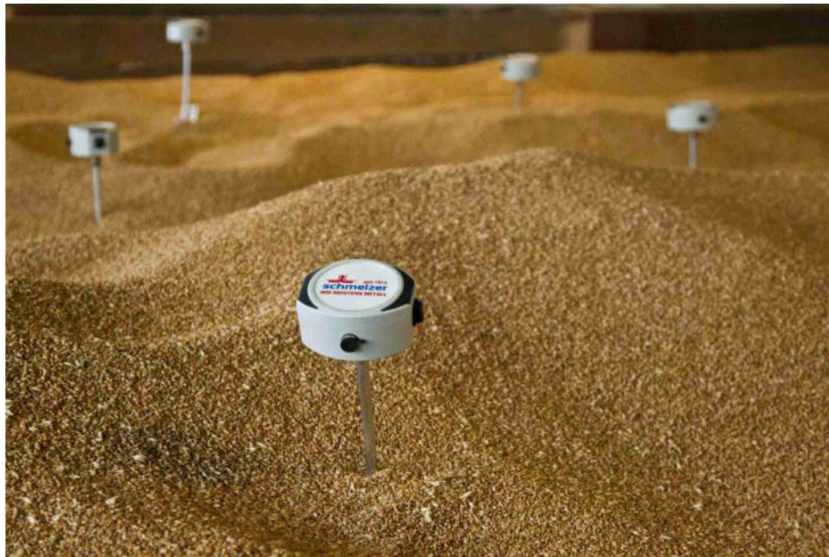
Figure 11: Measuring rods used in wheat.
