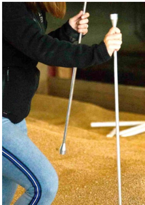
Figure 19: Insertion of the extension with tip into the bulk goods.
