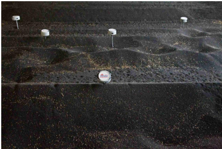
Figure 10: Measuring rods used in rape seed.
