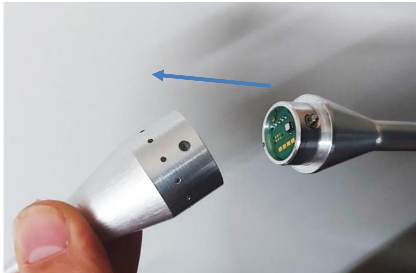
Figure 16: Removal of the measuring tip.
