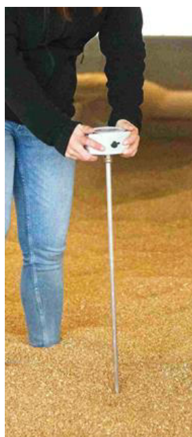
Figure 21: Measuring head must be set on top.
