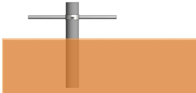
The fan is inserted in the Air lance (with help of a screwed connection). The sealing is fully automatically. Pay attention to the rotation of the engine after the device is connected to the mains (depending on the design). This is marked. The star delta combination contains a phase changer. If the rotation is wrong it has to be changed.
