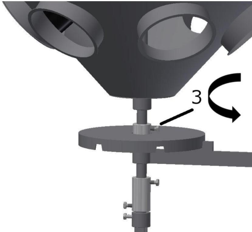
4. Now turn the inner tube so that it is above an outlet. Turn the turntable so that it clicks into place on the fixing lever.
