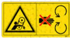
Do not open or remove protective device with the engine running!
