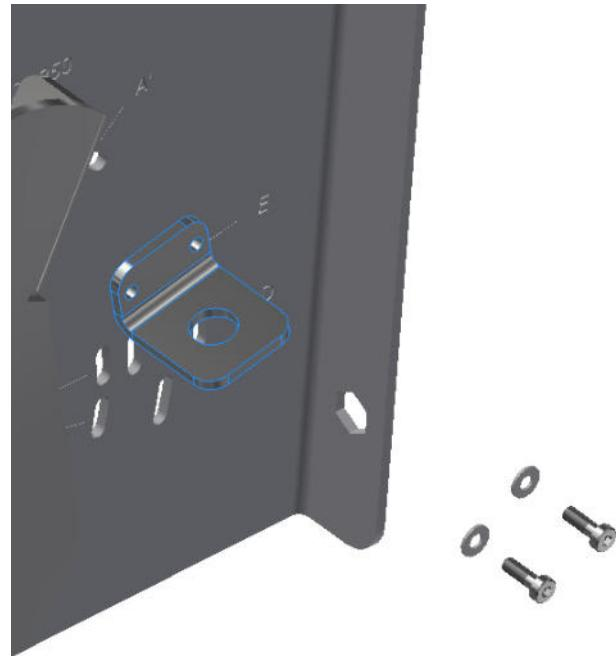
Use the screws provided to screw the limit switch bracket to the appropriate position.
