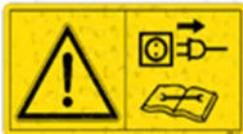
Before any cleaning, maintenance and repair work switch off the engine, pull the power plug or secure the main switch in zero position with padlock!
