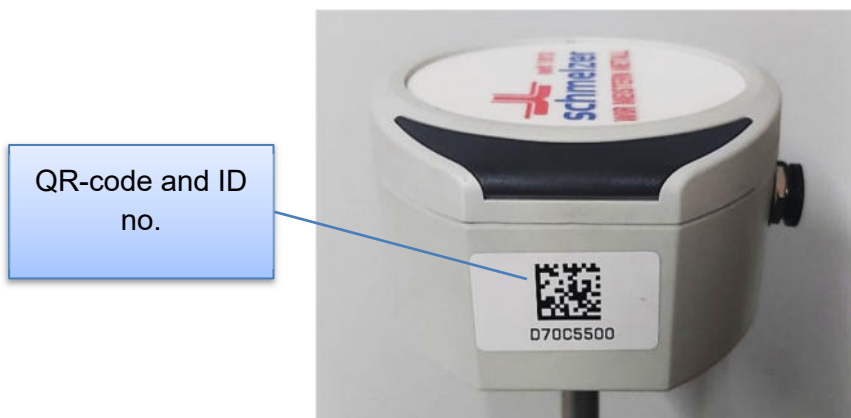
Figure 9: ID no. and QR-code on measuring head.
