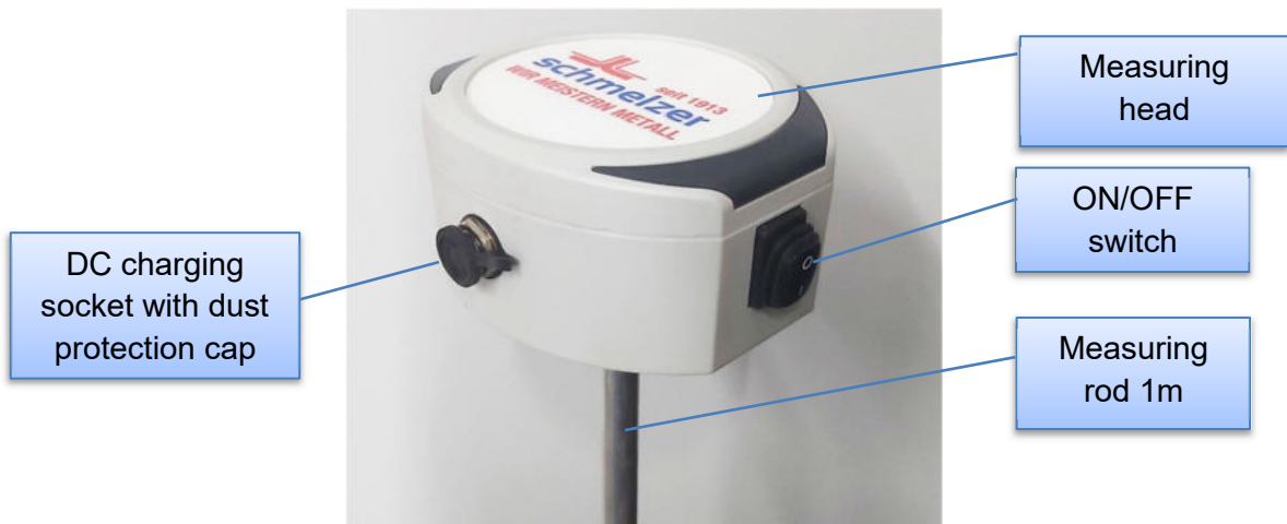
Figure 7: Measuring head overview
