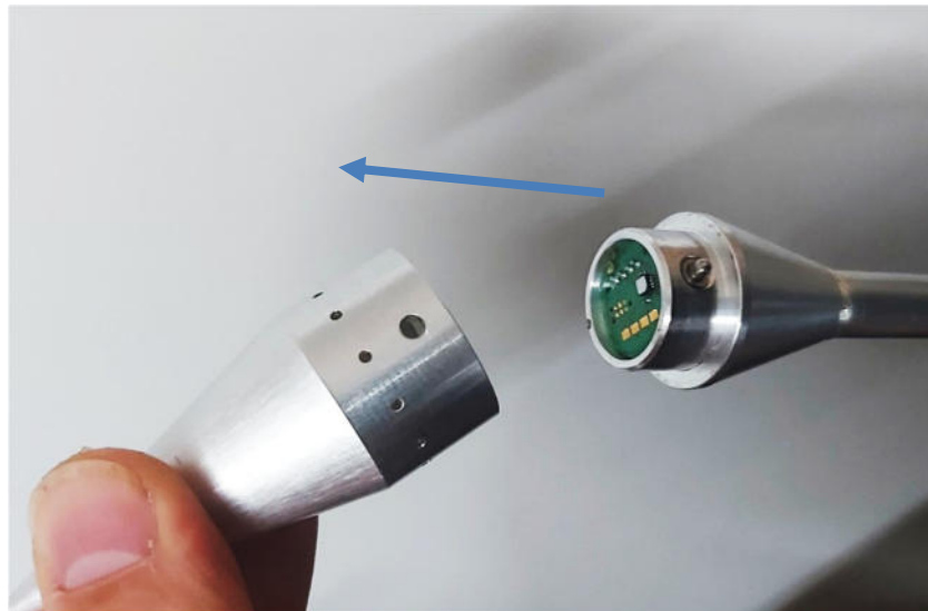
Figure 16: Removal of the measuring tip.
