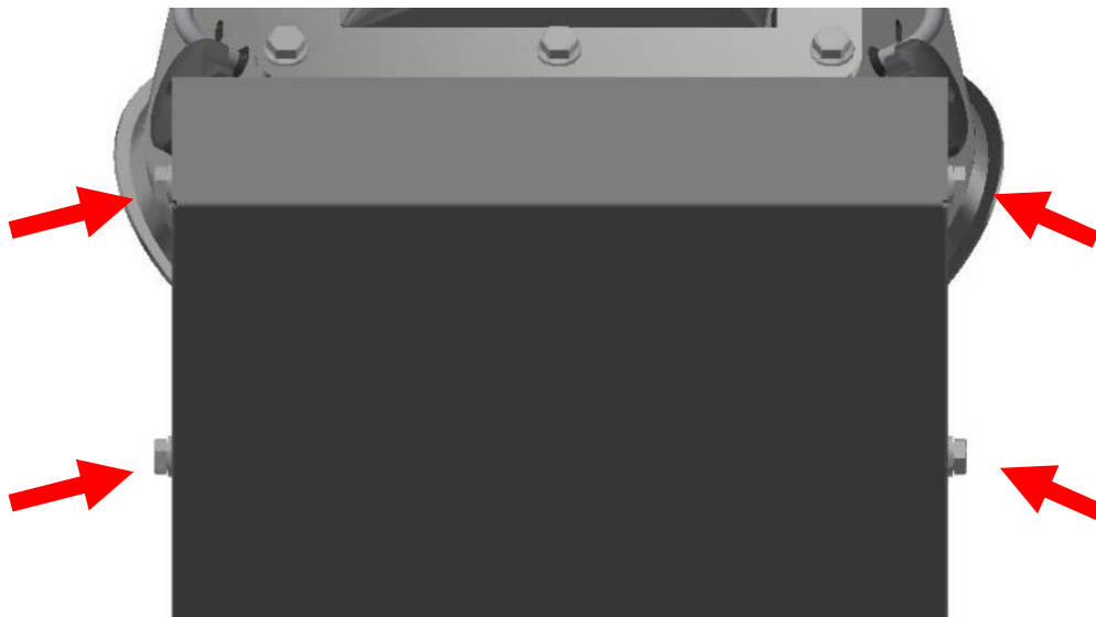
Figure 19: Disassembly of the cover for limit switches.
