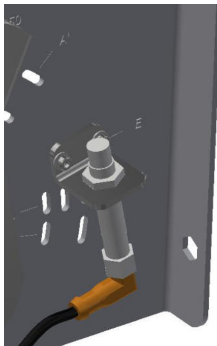
Figure 24: Setting the inductive limit switches.
