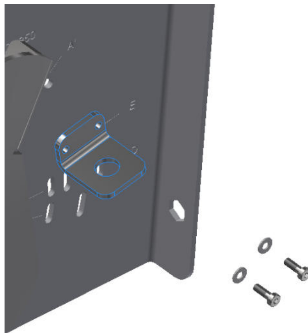
Figure 23: Installation of the bracket for inductive limit switches.
